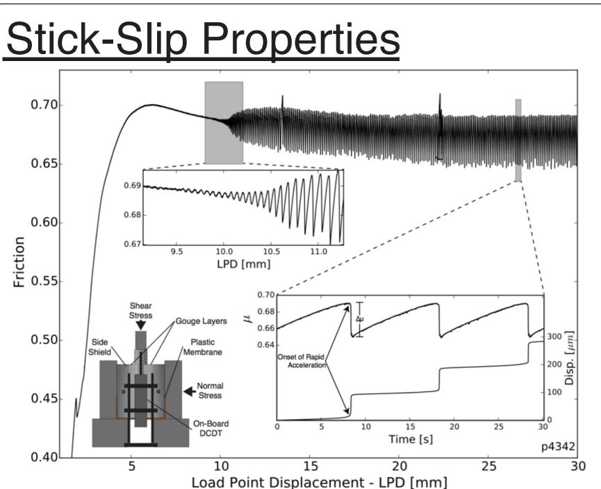
During the experiments, slow-slip events spontaneously emerge after ~10 mm shear displacement. The amplitude of the stick-slip events increases over a few millimeters of displacement, then reaches a steady value.
