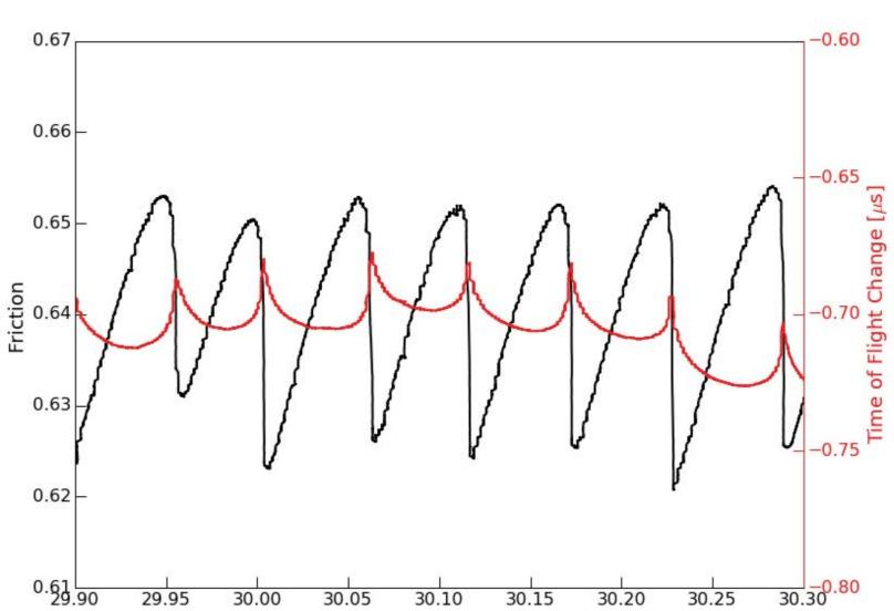
The acoustic time of flight (P-wave velocity) through the layers of fault gouge increases well before failure occurs, consistent with Kaproth and Marone (2013) and Scuderi et al., (2016). The results are also similar to observations of seismic velocity decreases before natural earthquakes.
