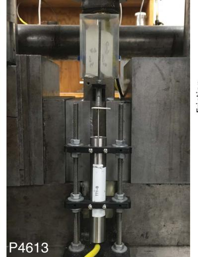
Most of the experiments shown were conducted by destiffening the shearing apparatus using an acrylic center forcing block (left). Similar results have been obtained by destiffening the system using an acrylic block as a spring above an all steel forcing block setup (right). Block wear is also much less of a concern using this technique.
