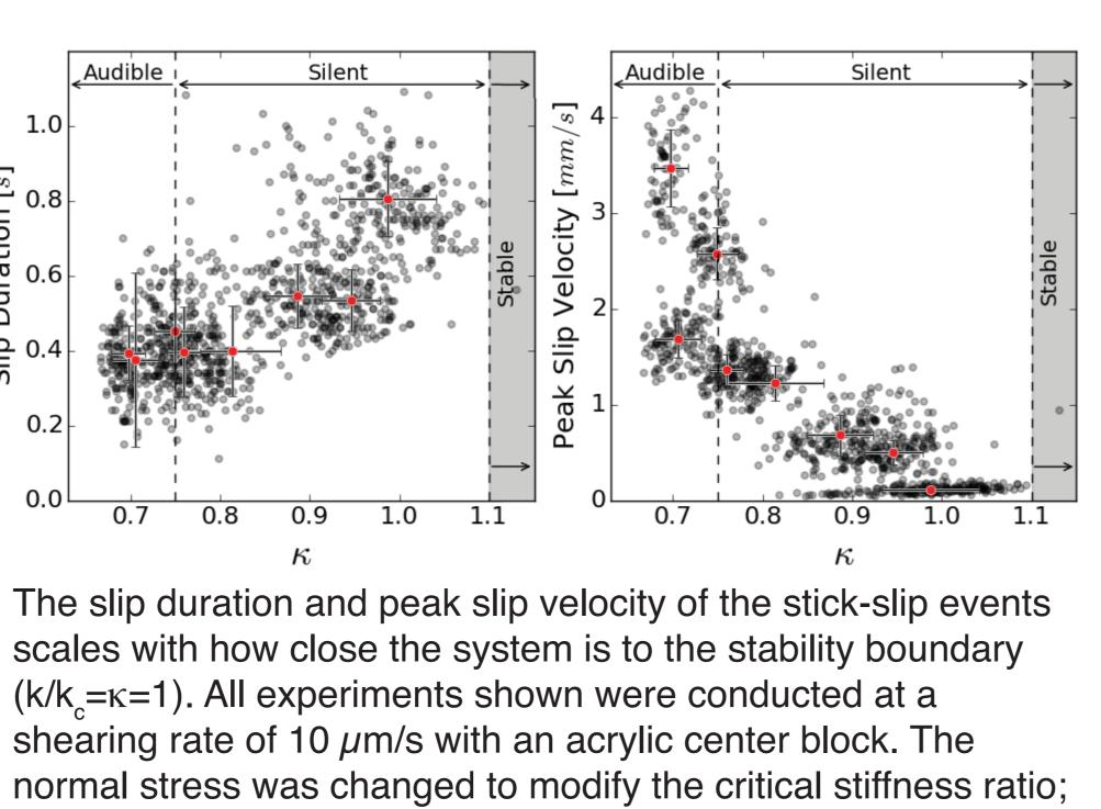
higher normal stresses push the system further into the unstable regime. The silent events are laboratory analogs of slow earthquakes, while audible events are considered regular earthquake analogs.
