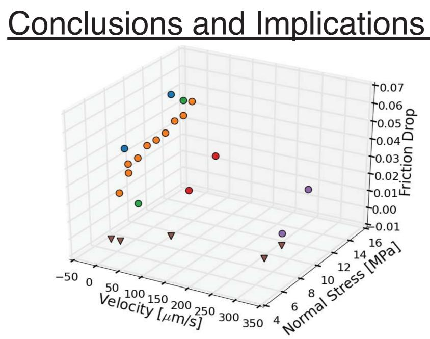
We have begun to map out the stability surface, showing that it is not simply a boundary between stable and unstable, but an envelope going from stable to growing stick-slip events. Triangles represent stable (zero friction drop) experiments. Each color is a constant shearing velocity.
