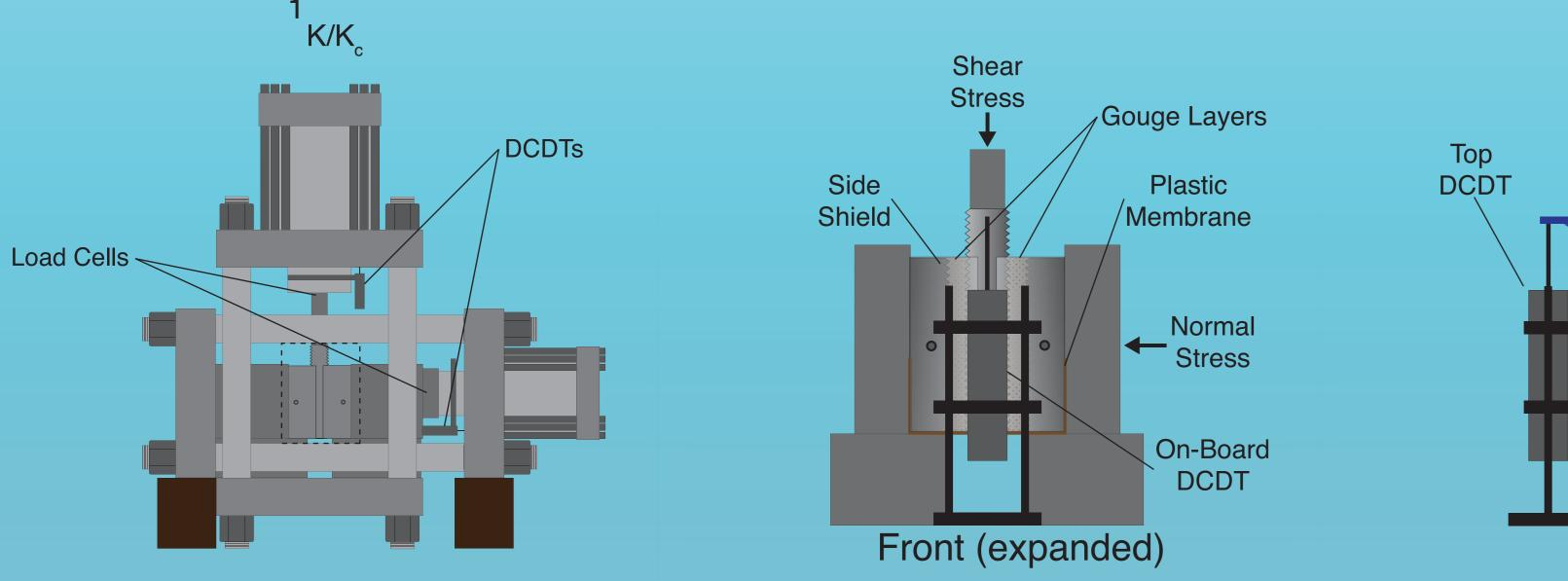
Samples were prepared using steel or titanium side blocks and steel or acrylic (PMMA) central shearing blocks. We used Min-U-Sil 40 powdered silica (U.S. Silica Co.) to simulate granular fault gouge. Samples were constructed as 3-mm thick layers, and with 10 cm x 10 cm frictional contact area. Layers were prepared and sheared under 100% relative humidity at room temperature.
