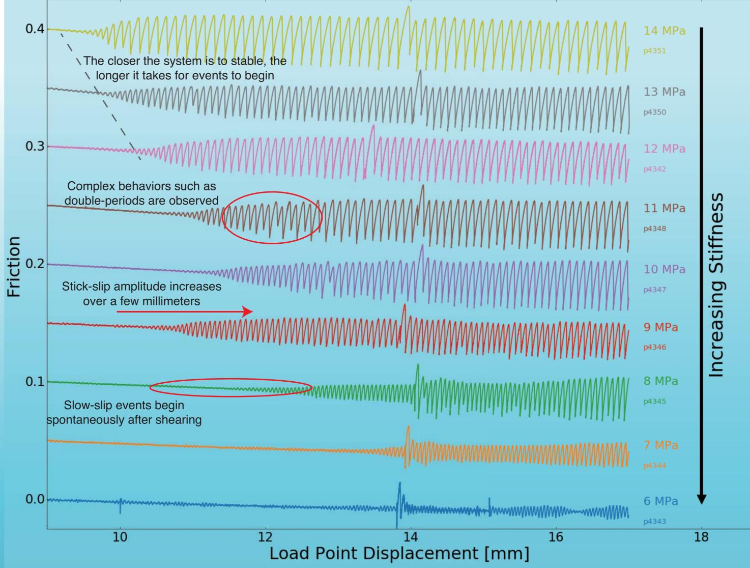
Experiments run at different normal stresses have different effective stiffnesses. Spikes are 13-14mm are holds while sensors were offset. We observe:
