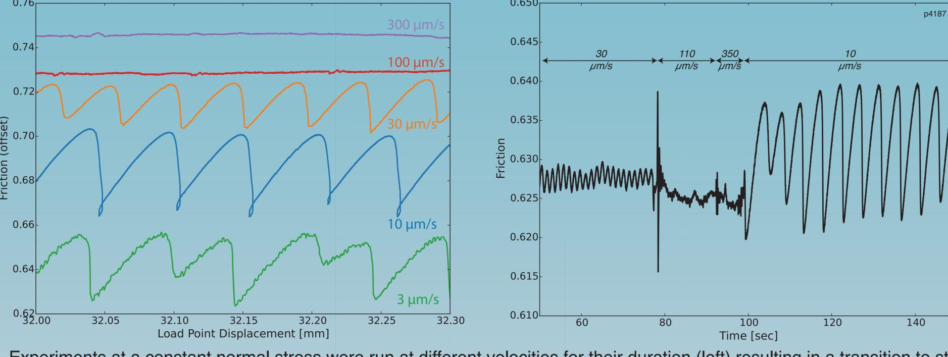
Experiments at a constant normal stress were run at different velocities for their duration (left) resulting in a transition to stable behavior at high driving velocities. In a similar experiment (right) we performed step changes to the velocity that turn on and off the slow-slip behavior. This indicates that either the system stiffness (k) or critical stiffness (k) is a function of velocity.
