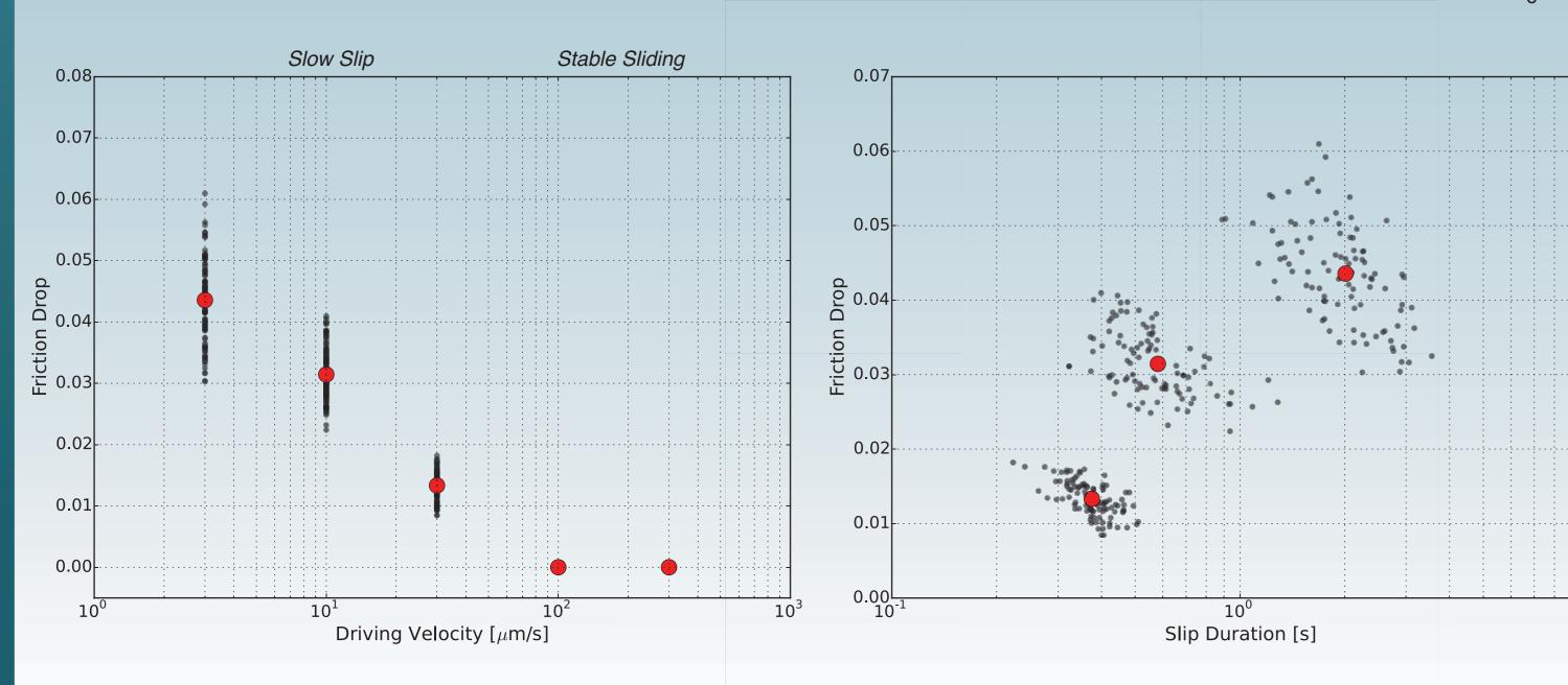
Friction drop and slip duration both show a systematic pattern with the driving velocity as has been observed for other laboratory stick-slip event catalogs. Data spread increases for lower slip rates and increasingly double period and complex behavior was observer. Non-linearity in slip-duration may be a function of how slip-duration is defined.
