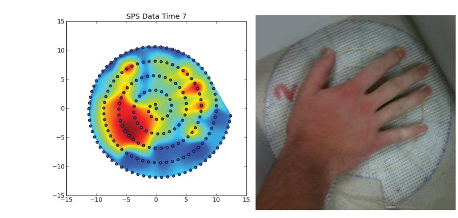
A hand placed on a LUNA DSS fiber produces a firm signature in the temperature contour plot.
