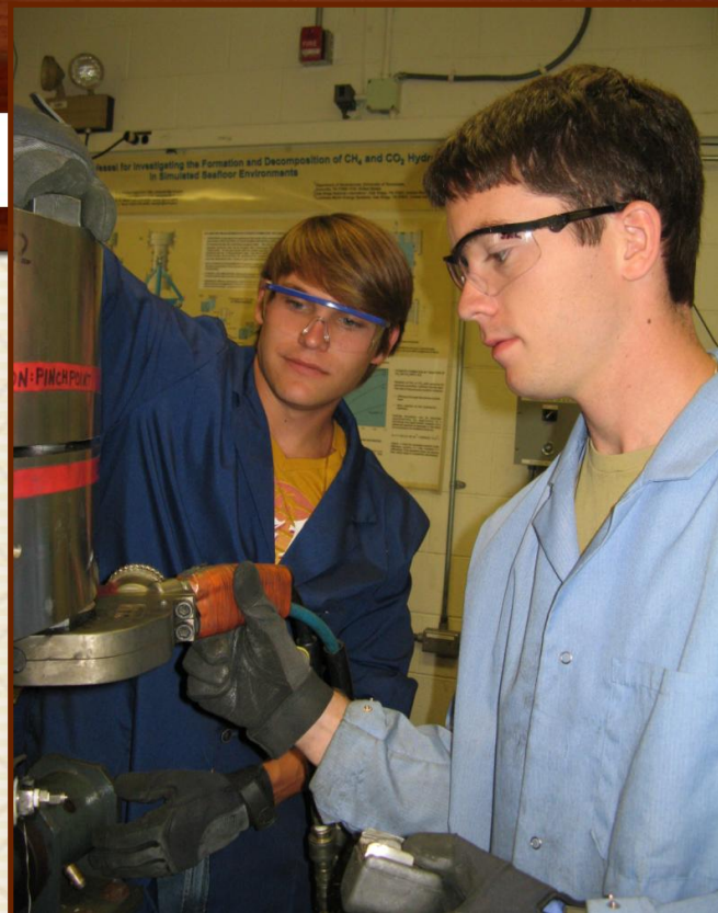
Title Figure: Sealing the lid of the SPS with a hydraulic torque wrench.
