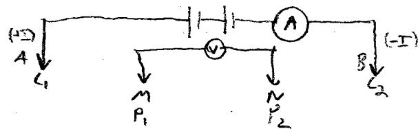
We input power and measure its current at electrodes A + B and measure the potential difference across M + N
