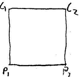
This gives us easy gridding and by swapping P<sub>1</sub>, P<sub>2</sub> we get an orthogonal reading for resistivity anisotropy.
