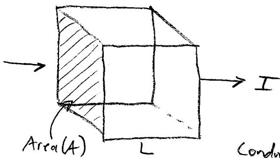
Passing current through this cube of resistive material we can see resistivity is proportional to length and inversely proportional to cross sectional area
